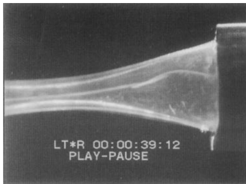
Figure 2. Flow attached to one side of the tube-divergent nozzle.
